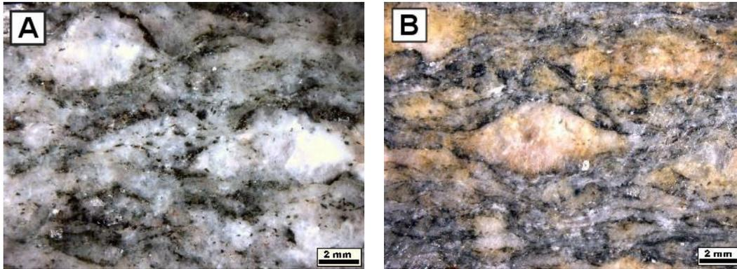
**Fig. 3: Macrographs of Luserna Stone varieties: A: Massive facies; B: Splittable facies (samples before crushing test) (Vola et al., 2008).**
