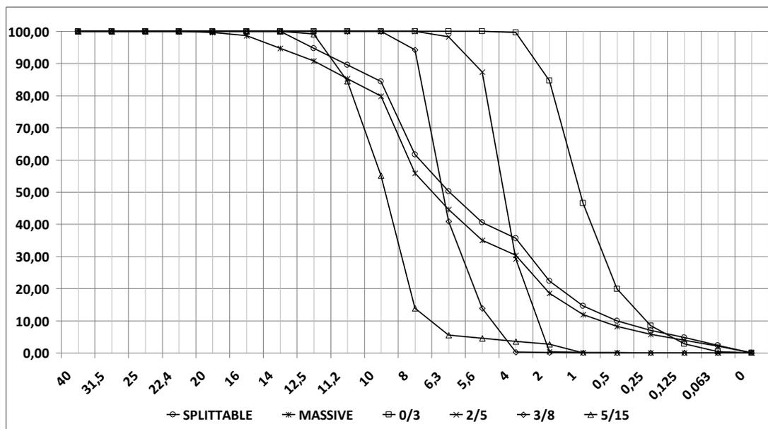
**Fig. 4: Particle-size distribution curves of Luserna fractions**
