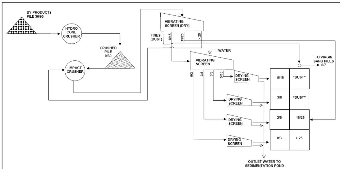
**Fig. 2: Flow sheet of the crushing and screening plant used for the industrial test at “Cava Monviso”, Casalgrasso, Cuneo.**
