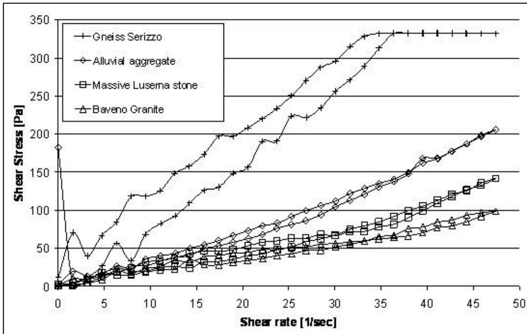
**Fig. 6: Rheological curves of mixes with different aggregates.**
