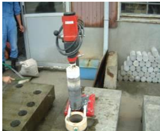
Fig. 2. Overview of drilling cores from specimens exposed outdoor
