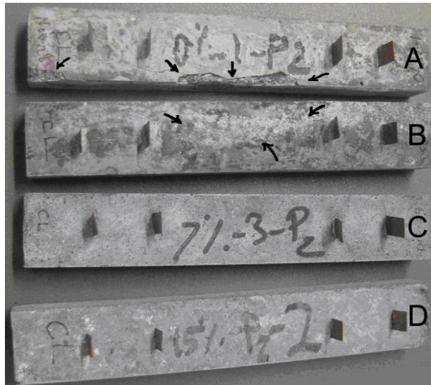
Figure 7. Effect of chloride solution on the appearance of the specimens (A: 0% CF; B: 3.5% CF; C: 7% CF; D: 15% CF)
