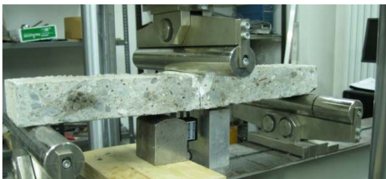
Figure 1. Three-point bending test set-up
