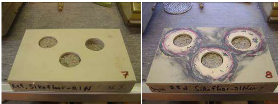
Figure 2. Test slabs with system 5G after pull-off testing, without exposure (left hand picture) and after exposure (right hand picture)
