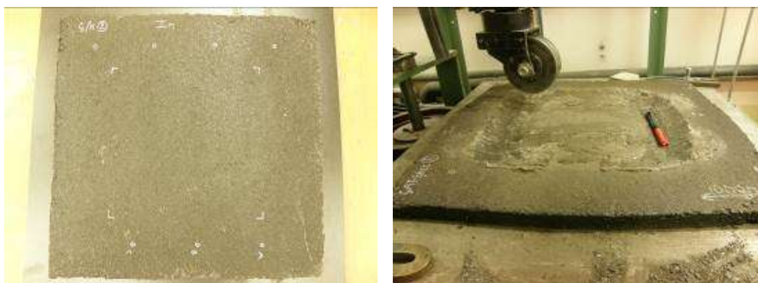
Figure 3. Test slab of PGJA before and after testing according to EN 13892-5
