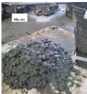
(a) Collapse type.
