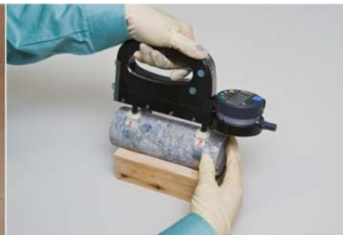
Figure 2 Measurement of the expansion of the core
