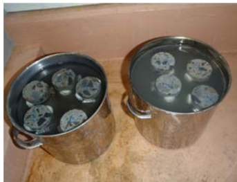
Figure 1 Cores immersed in a 1N-NaOH
