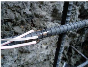
Figure 3 Setting up of strain gauges
