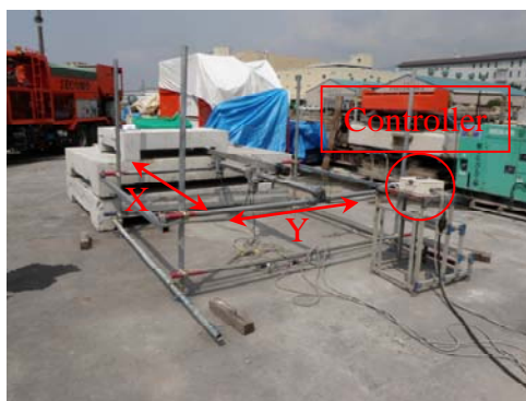
Photo 3. Water jet robot
