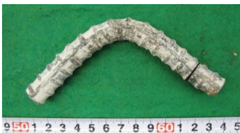
Figure 11. Steel bar used in measurement of bending radius (D16)
