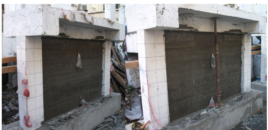
a) R , with a non-loaded panel b) SPI , with a pre-loaded panel
