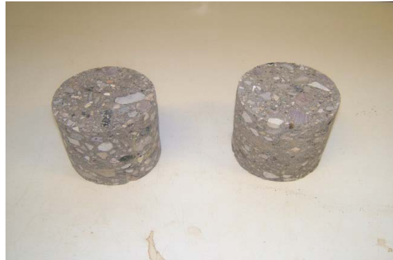
Figure. 5 Cores from trial of roller compacted concrete with CEM0 and crushed concrete aggregate used in a car park.
