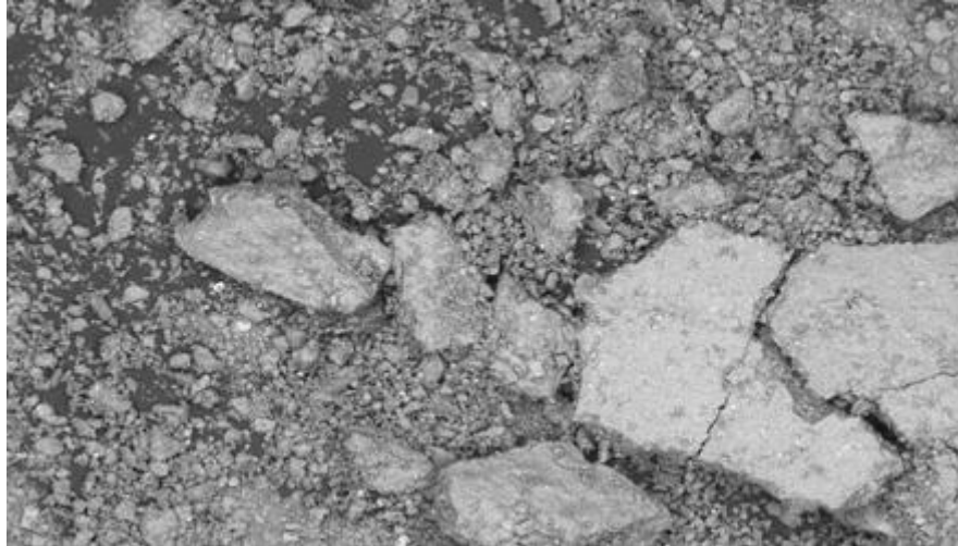
Figure 8. The Scanning Electron Microscope (SEM) of kaolin clay (alafya) after treatment.
