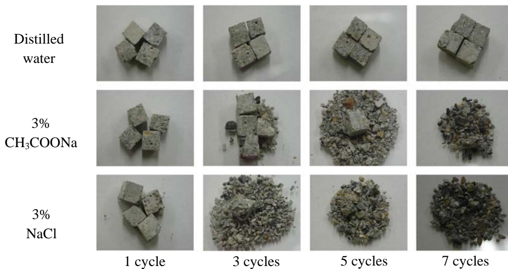
Figure 2 Appearance of specimens as the freeze-thaw test cycling progressed.
