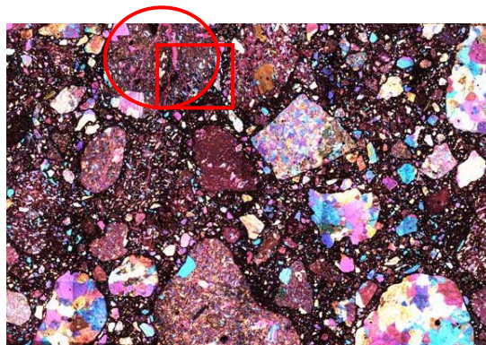
Photograph 2. Composite pictures of entire thin core sections (OPC, interior of the core, Optical microscope image under crossed nicols)
