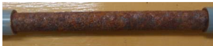
Photo 2. Corrosion of test piece
