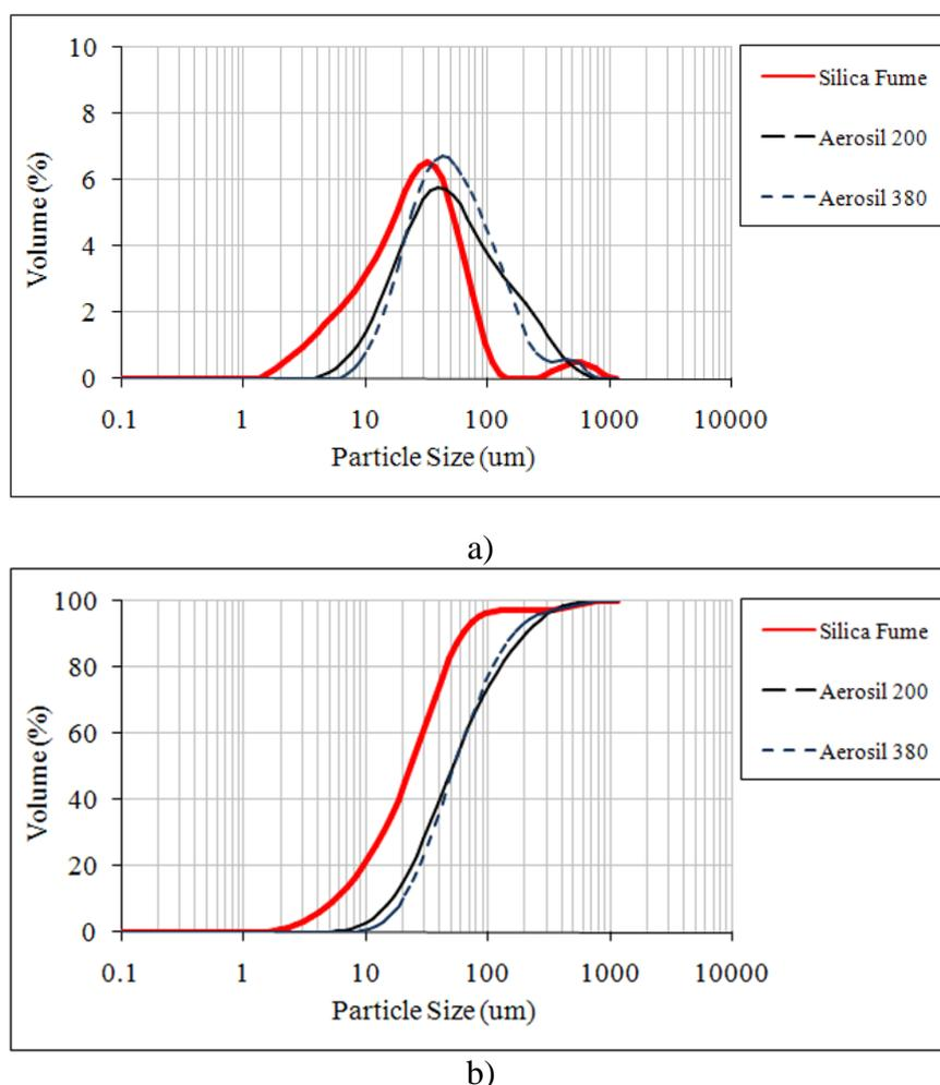
Fig 4. Size distribution of the pyrogenic nanosilicas and silica fume under low shear mixing with water for 4 min a) non-cumulative and b) cumulative
