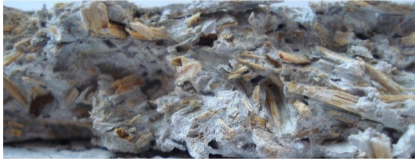
Figure 18. Detail of sample structure by formula C09-10 (fracture area after bending strength test)
