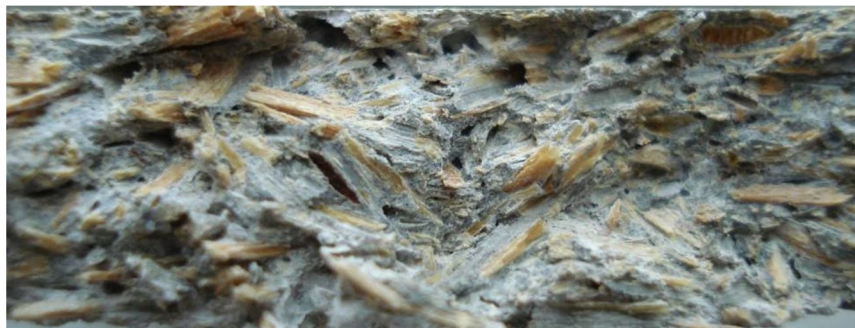
Figure 17. Detail of sample structure by formula REF (fracture area after bending strength test)
