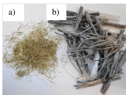
Figure 1. Fibers: a) steel flat ( S ) 6 mm, b) structural polypropylene ( R ) 54 mm
