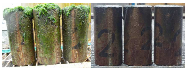
Photo 1. Specimens after 5 years exposure (HHS-1, left: splash zone, right: tidal zone)
