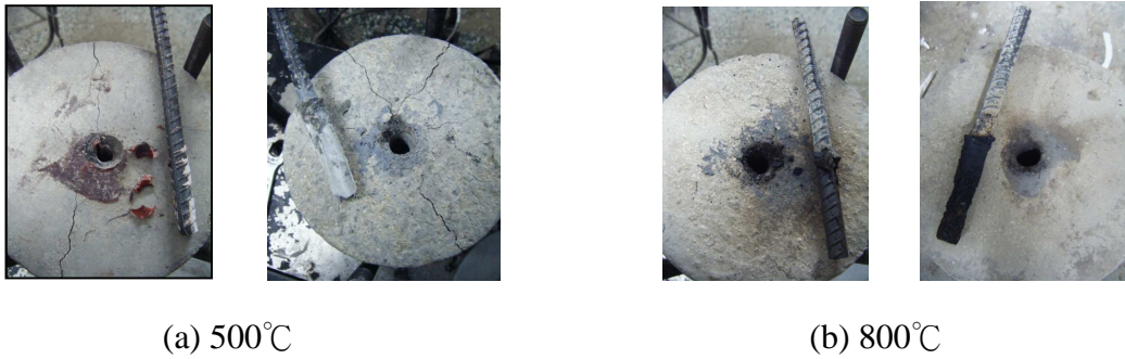
Figure 5 Bond failure of pull-out test
