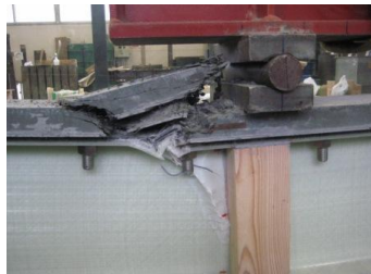
(a) Crushing of UHSFRC slab
