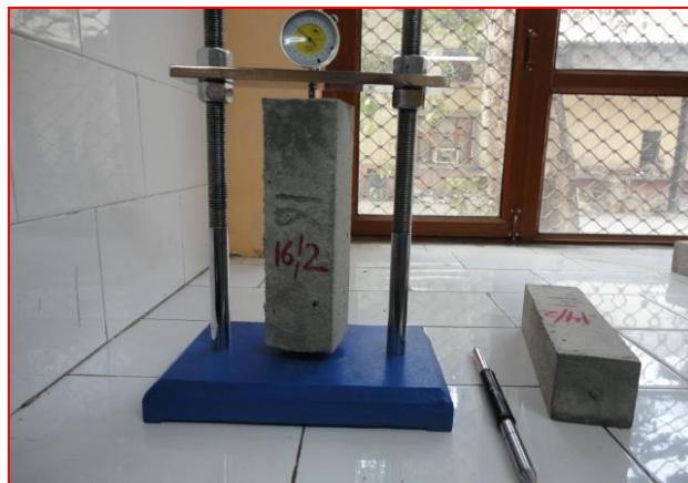
Figure 2. A concrete specimen under drying shrinkage test
