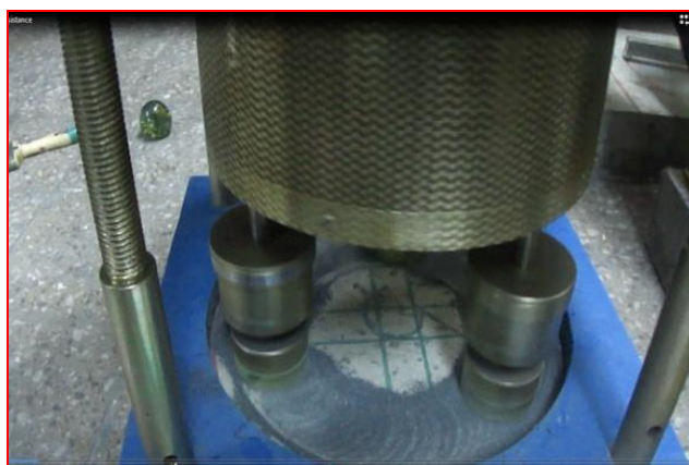
Figure 3. A concrete slab under abrasion testing
