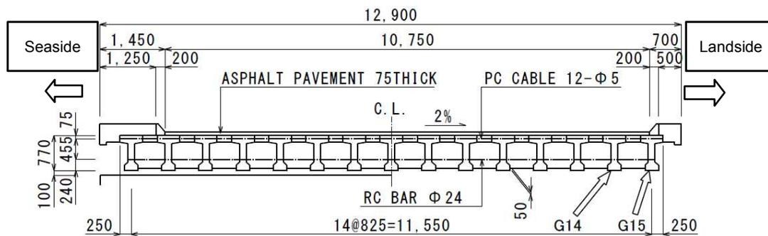
Figure 1. Outline of Removed Road Bridge (Unit : mm)
