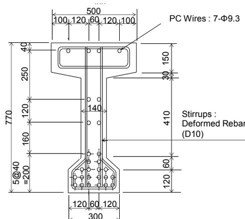
Figure 2. Cross-Section of PC Girder (Unit : mm)
