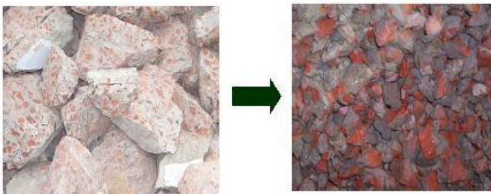
Figure 1. Demolished concrete block and recycled aggregates
