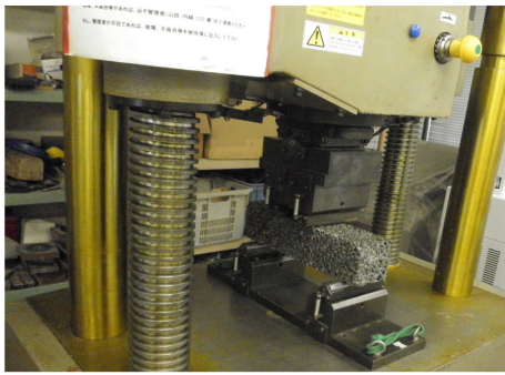
Fig. 4 Flexure strength test
