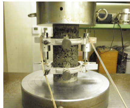
Fig. 5 Compression strength test and modulus of elasticity measurement Flexure strength test
