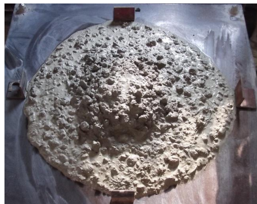
Photo 2. An example of segregated flowable concrete
