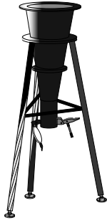
Figure 5. Outline of funnel flow time test of concrete
