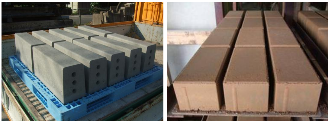
Figure 2. Appearance of new ecological concrete (left) and mortar (right)
