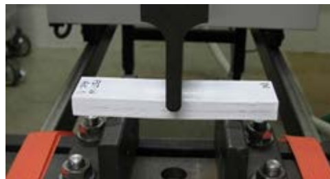
Figure 3 Interlaminar shear test of flange specimen
