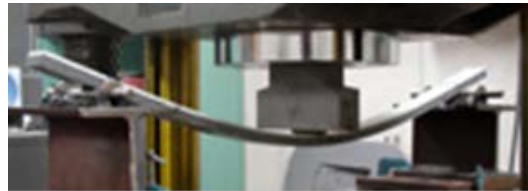
Figure 2 Bending test of flange specimen
