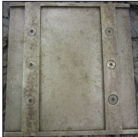
Figure 1. Steel mould (Internal dimension: 200×100× 5 mm)
