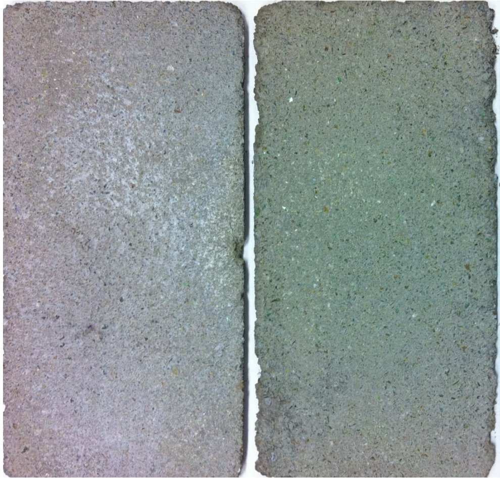
Figure 6. Photograph of Spray AB (left) and 5%TiO 2 intermixed surface layer (right) undergone 100 times abrasion
