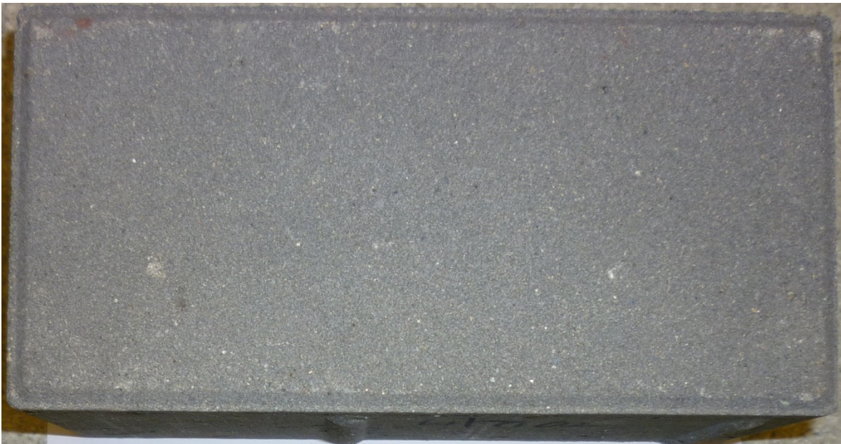
Figure 2. Concrete block used to apply the abrasion load
