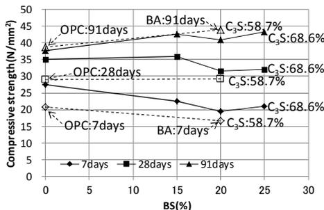
**Fig.7 Relationship between BS content and compressive strength ( $10C^\circ$ )**
