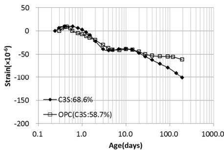
**Fig.9 Test results of autogenous shrinkage (BS: 0%)**
