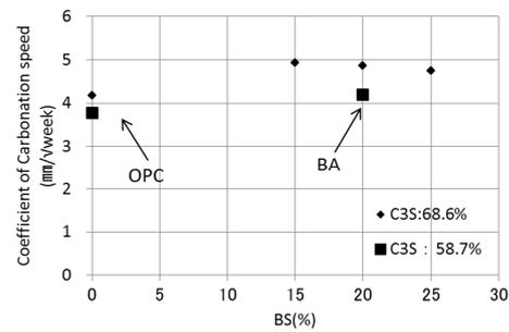
**Fig.18 Relationship between BS content and coefficient of carbonation speed**
