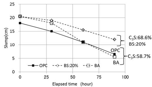
**Fig.1 Change in slump with time**
