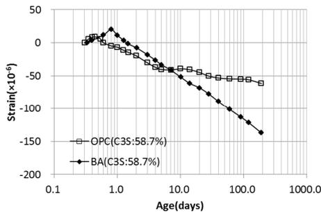
**Fig.11 Test results of autogenous shrinkage**
