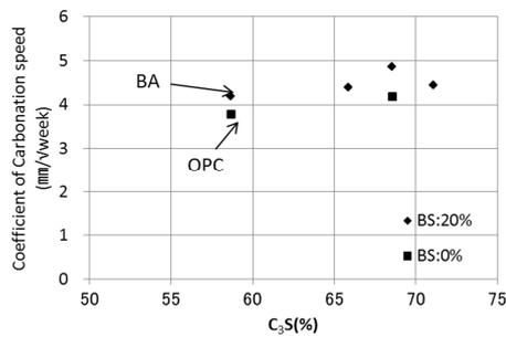
**Fig.17 Relationship between C<sub>3</sub>S content and coefficient of carbonation speed**
