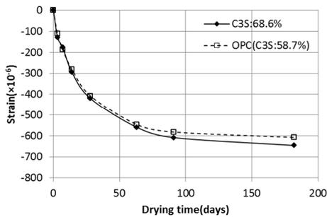
**Fig.13 Test results of drying shrinkage (BS: 0%)**
