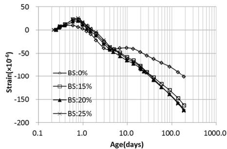
**Fig.12 Test results of autogenous shrinkage ( $C_3S$ : 68.6%)**
