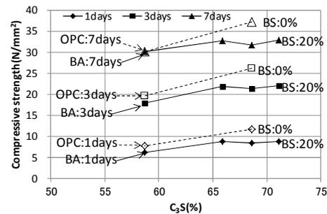
**Fig.4 Relationship between  $C_3S$  content and compressive strength ( $20C^\circ$ )**
