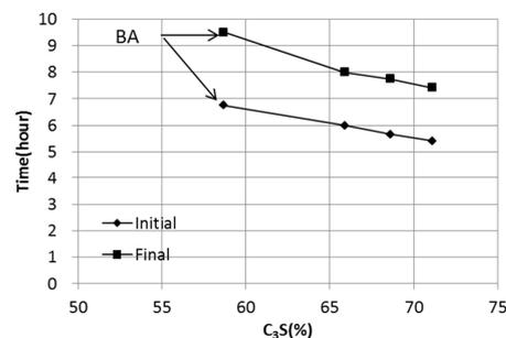
**Fig.3 Relationship between C<sub>3</sub>S content and setting time (BS : 20%)**
