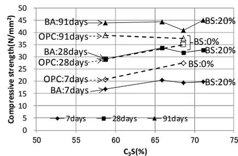
**Fig.6 Relationship between  $C_3S$  content and compressive strength (BS: 20% , $10C^\circ$ )**
