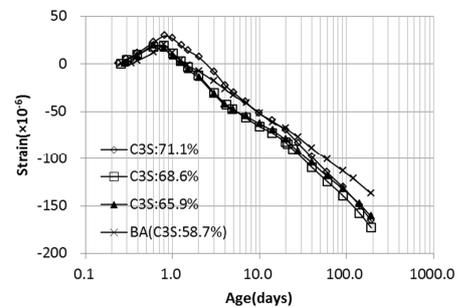
**Fig.10 Test results of autogenous shrinkage (BS:20%)**
