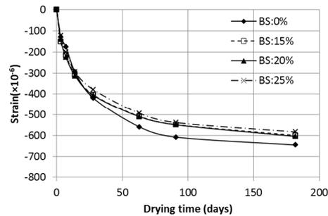
**Fig.16 Test results of drying shrinkage ( $C_3S$ :68.6%)**
