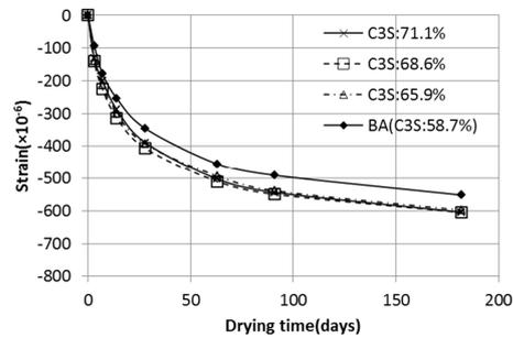
**Fig.14 Test results of drying shrinkage (BS: 20%)**
