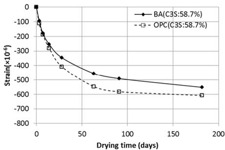
**Fig.15 Test results of drying shrinkage ( $C_3S$ :58.7%)**
