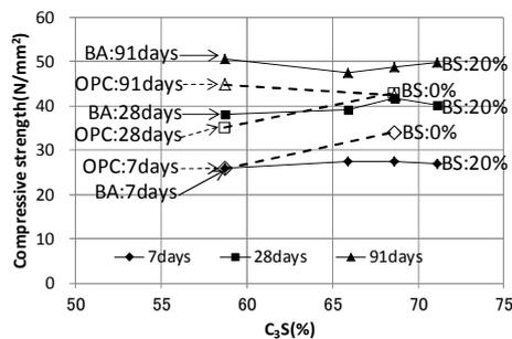
**Fig.5 Relationship between  $C_3S$  content and compressive strength (BS: 20% , $20C^\circ$ )**
