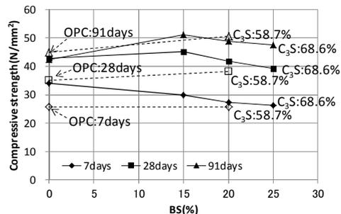
**Fig.8 Relationship between BS content and compressive strength ( $20C^\circ$ )**
