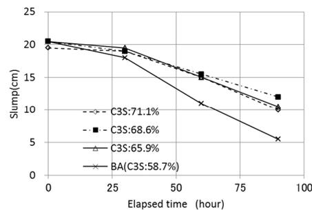
**Fig.2 Change in slump with time (BS : 20%)**
