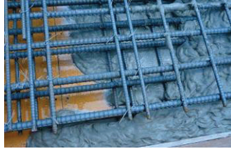
Photo 4. Flow Condition within the Test Piece Form
