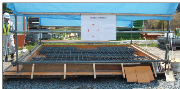
Photo 3. Full View of the Slab-imitating Test Piece
