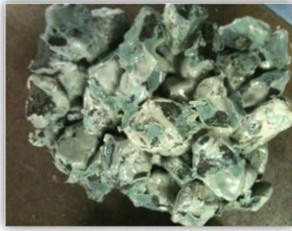
Fig. 6. sections that were destroyed by the strength tests
