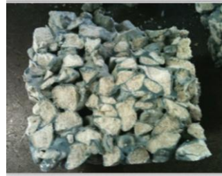
Fig. 6. sections that were destroyed by the strength tests
