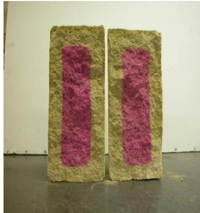
Figure 1. Test Cylinder Treated with Indicator Solution
