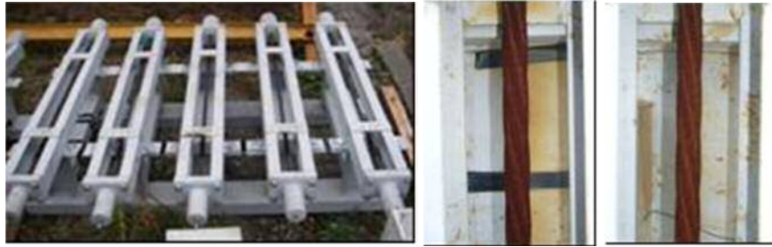
Figure 9. The appearances of prestressing strands after 440 days of outdoor exposure test (left; test status, center; high-strength prestressing strand, right; conventional prestressing strand)
