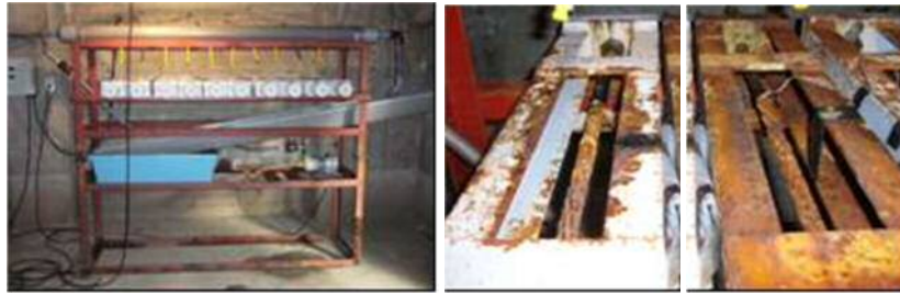
Figure 11. The appearances after 440 days of wet-dry cyclic test (left; test status, center; HPS, right; CPS)
