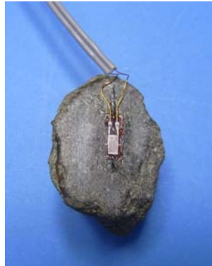
Figure 1. Measurement method for shrinkage of aggregate
