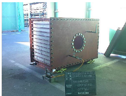
Figure 8. Supporting members to keep water tightness
