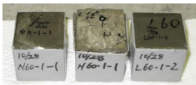
Photo 1. External appearances after 12 weeks (OPC60, HPC60 and LPC60)
