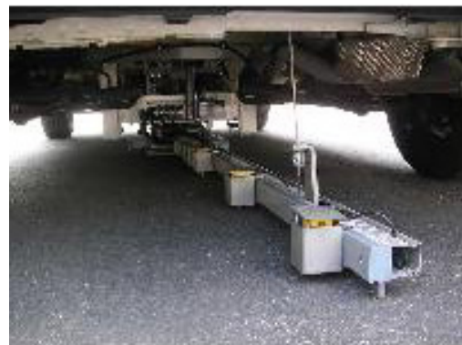
Fig.5 Displacement sensor mounted in FWD testing vehicle 4)
