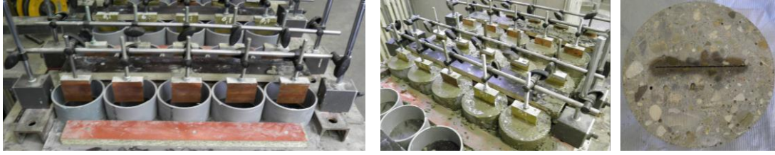
Figure 2. Positioning of the steel plates (left), Casting of the samples (middle), Prepared concrete sample (right).
