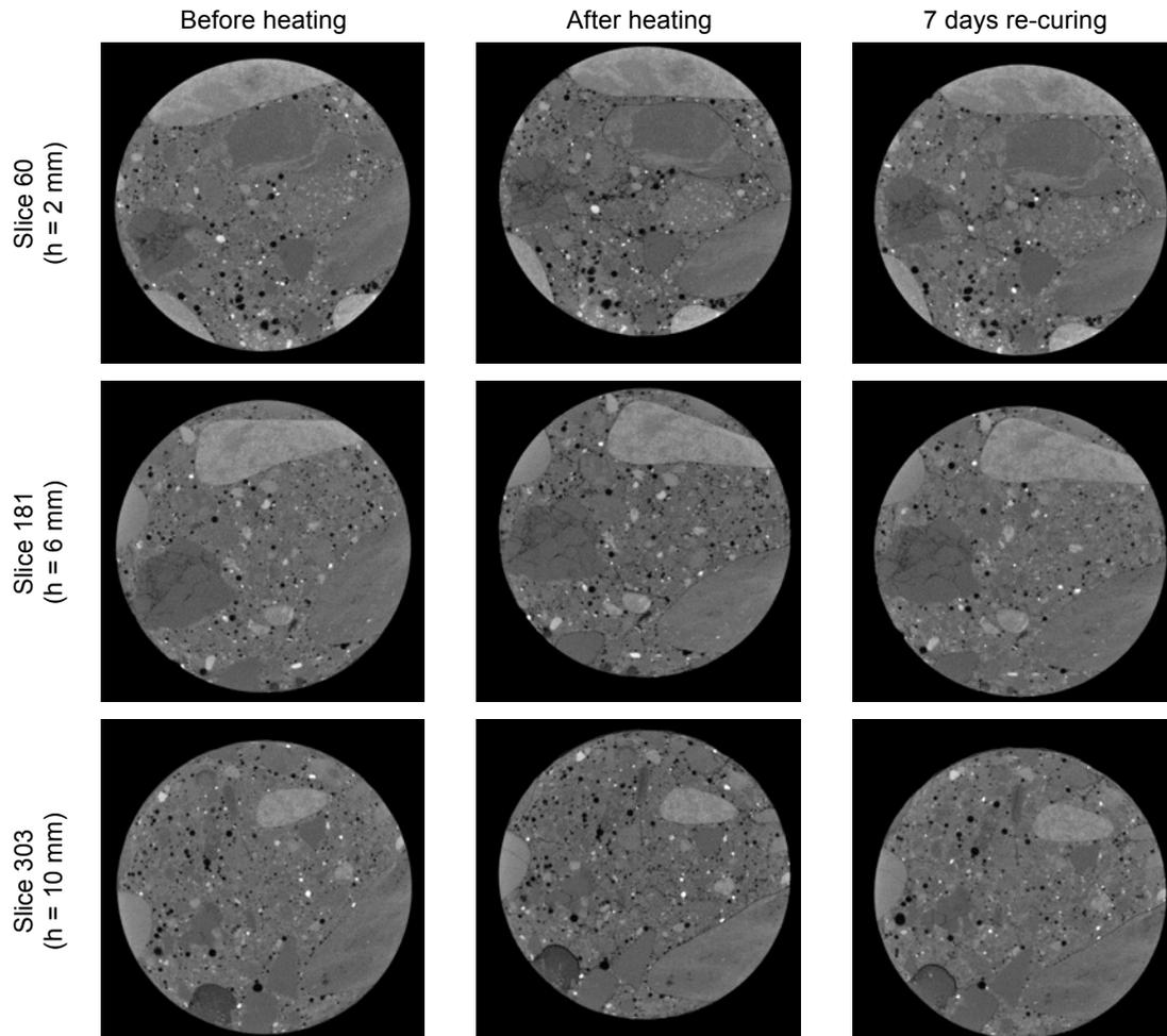
**Figure 5. Cross sections at various heights of concrete specimen**
