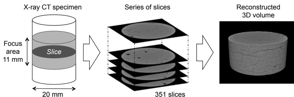
**Figure 3. Details of X-ray CT specimen and 3D digital image reconstruction**
