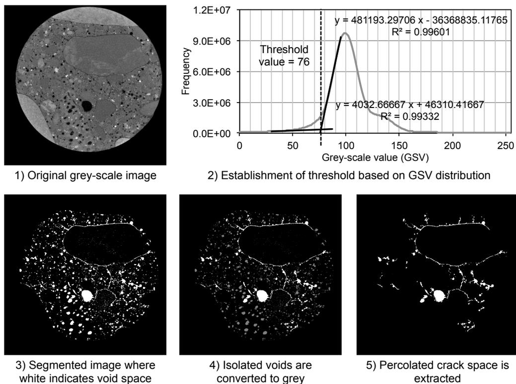
**Figure 8. Method of segmentation for identifying percolated crack space**
