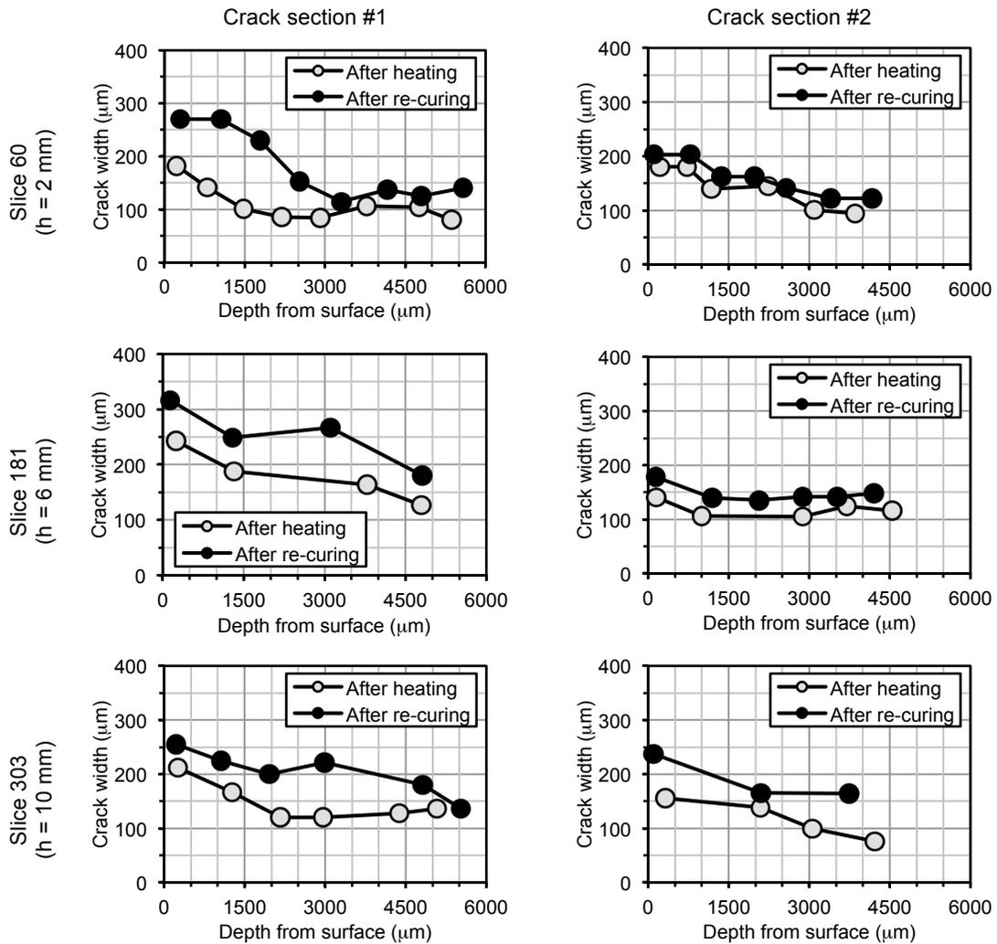
**Figure 7. Change in crack width from surface for selected crack sections at various heights of cement paste specimen**
