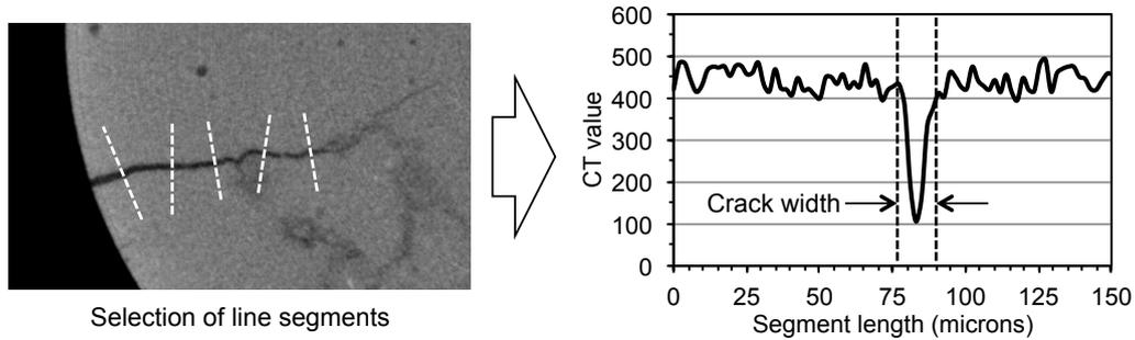
**Figure 6. Method of calculating crack width**
