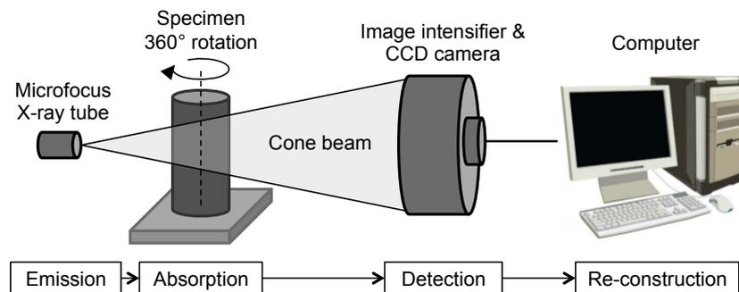
**Figure 2. Set-up for X-ray CT image acquisition**
