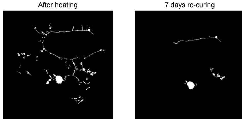
**Figure 9. Comparison of percolated crack space in concrete specimen**
