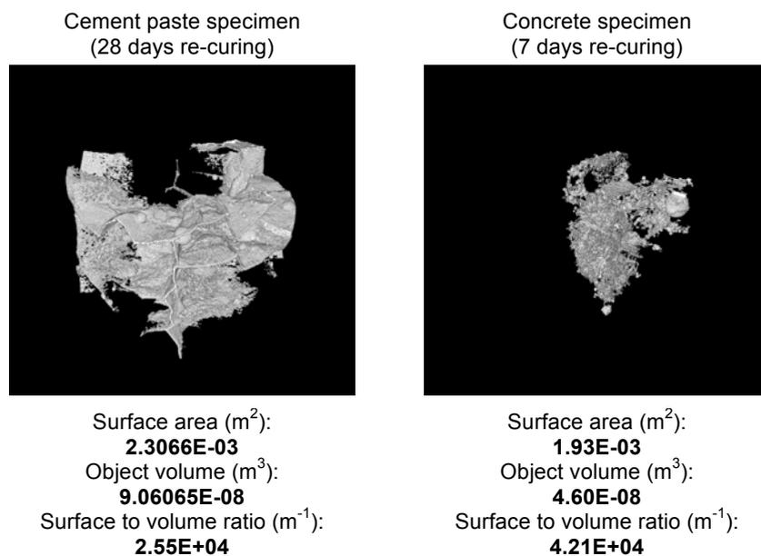
**Figure 10. Comparison of 3D crack volume and characteristics after re-curing**
