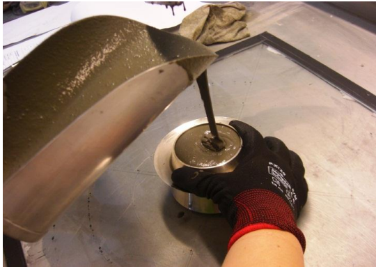
Figure 3. Slump flow test of UHPFRC mixture
