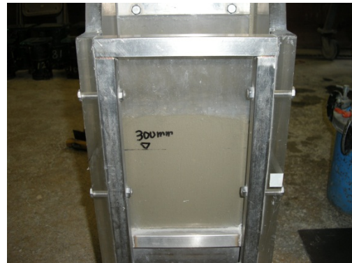
Photo 2 – Result of U-Box test (R2)
