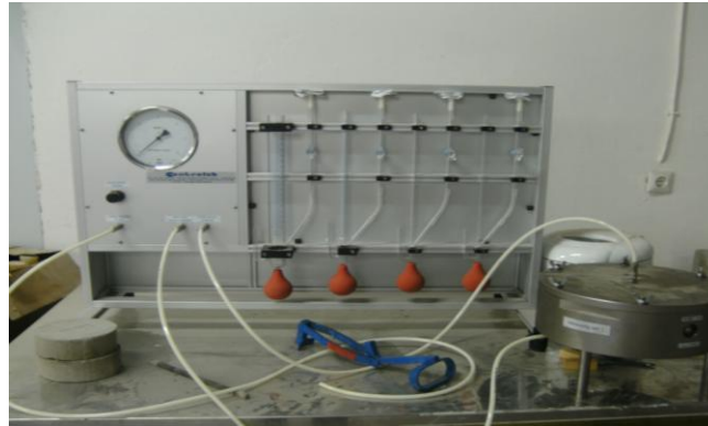
Figure 3. Air permeability test equipment
