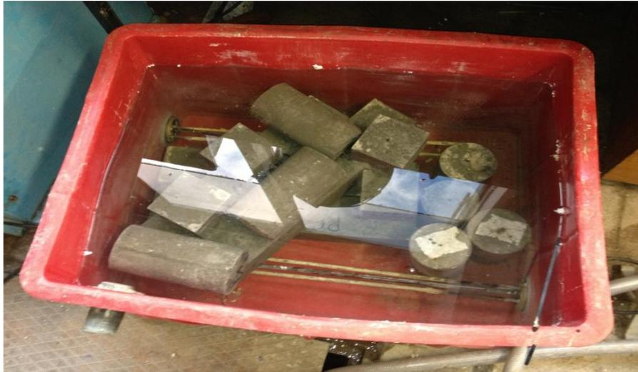
**Figure 1. Hot curing of concrete specimens**
