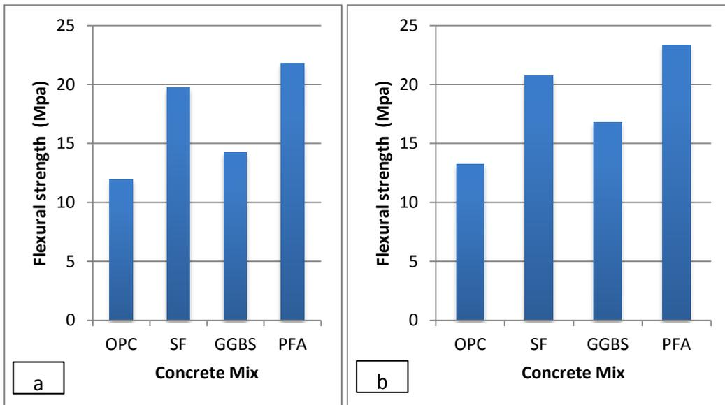
**Figure 8. Comparison of flexural strength a) before and b) after accelerated corrosion**
