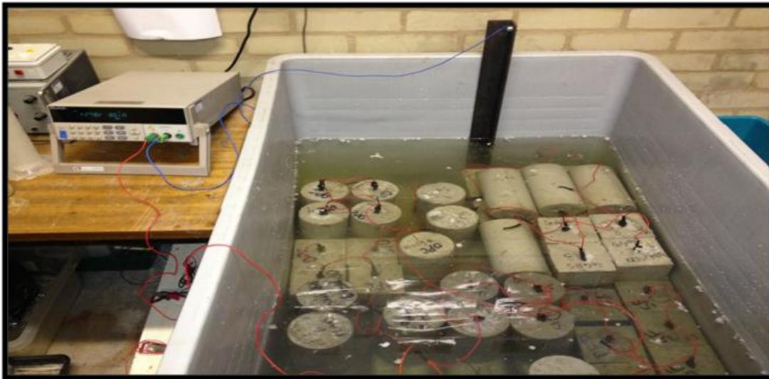
**Figure 3. Corrosion tank used for accelerated corrosion test**
