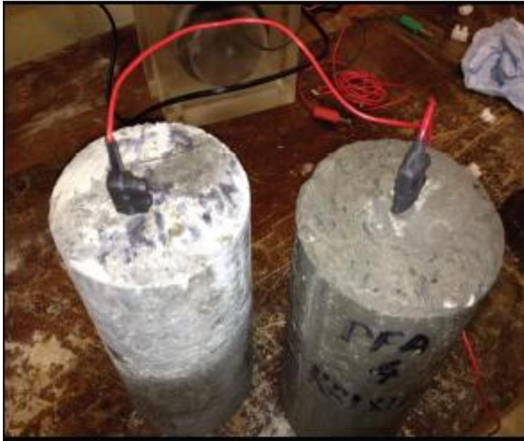
**Figure 4. Concrete specimens before accelerated corrosion test**
