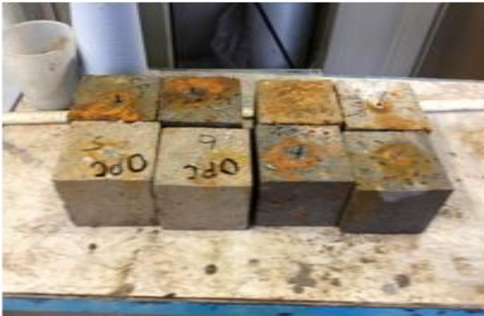
**Figure 5. Concrete specimens after accelerated corrosion test**
