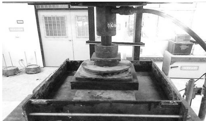
Figure 3. Molding system set with 20 tonne hydraulic pressure
