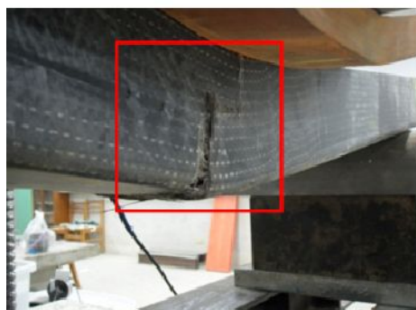
Figure 8. The failure mode of specimen BDEM
