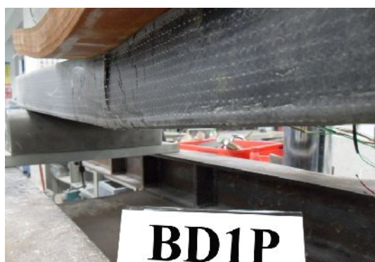
Figure 2. Failure mode of BD1P from three-point bending test at the web
