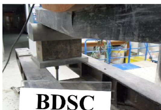
Figure 4. The failure mode of specimen BDSC from three-point bending test
