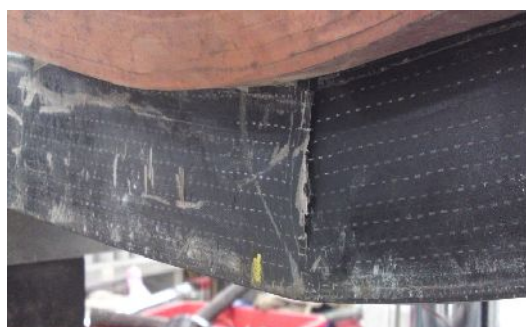
Figure 6. The failure mode of BDNC from three-point bending test
