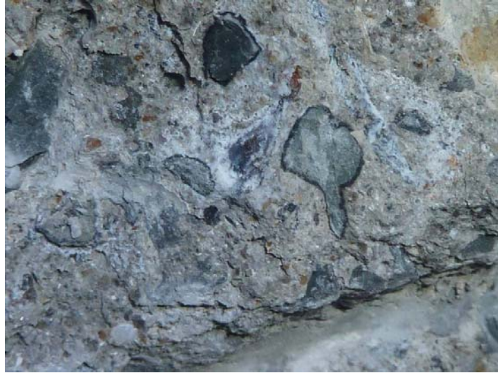
Figure 8. The gel and the reaction ring observed in P369 concrete
