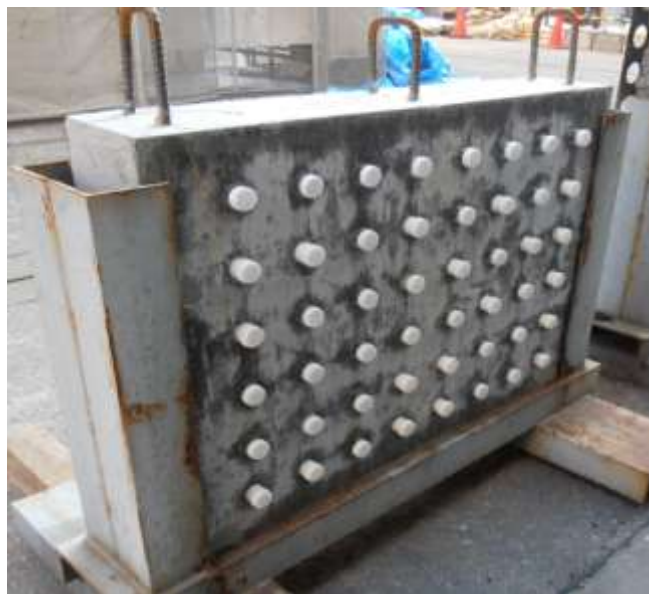
Photo 2. Concrete panel specimen embedding PET bottles
