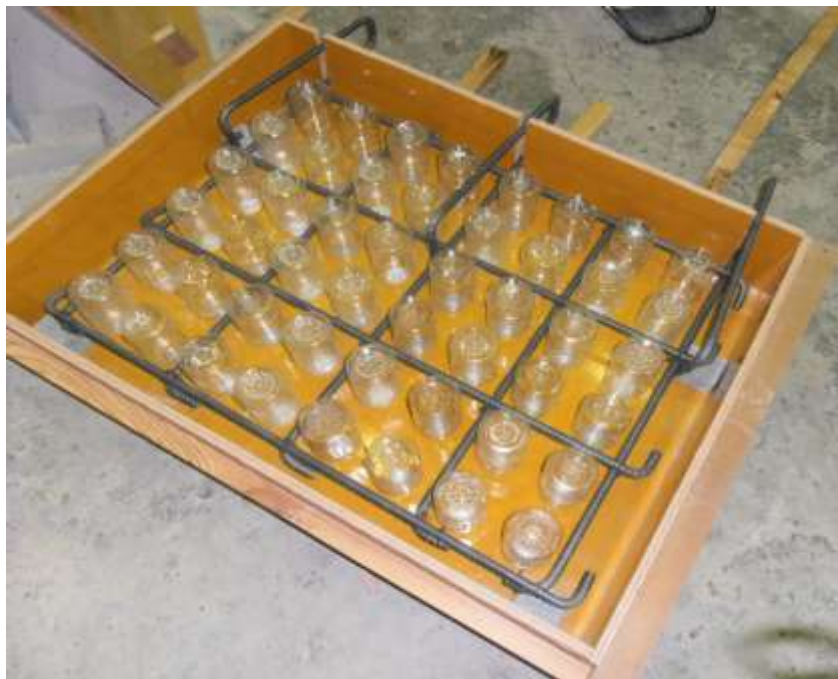
Photo 1. PET bottles fixed in the mold
