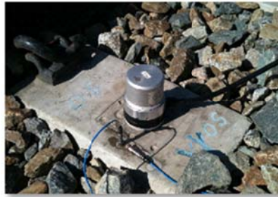
Figure 5. Geophone and Accelerometer
