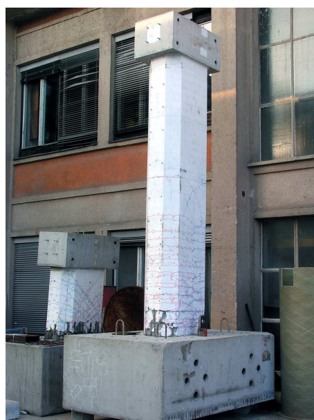
Figure 2: Short and high column models after finished experiments
